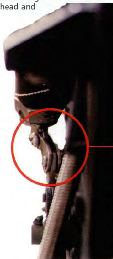
(Left) The ejection-seat guillotine linkage was bent when someone forced the seat up while the lap belt was wedged between the seat and the bulkhead.
